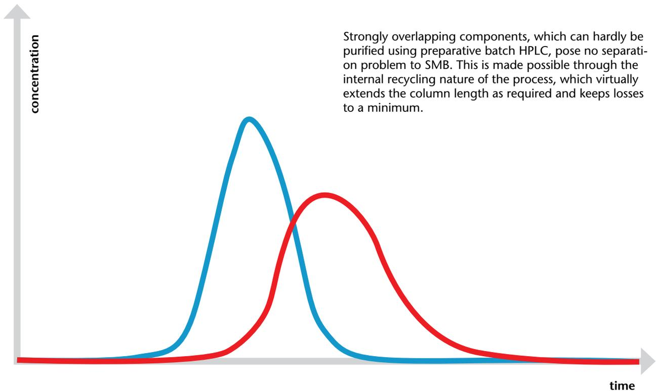
Strongly overlapping components, which can hardly be purified using preparative batch HPLC, pose no separation problem to SMB. This is made possible through the internal recycling nature of the process, which virtually extends the column length as required and keeps losses to a minimum.
