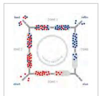
Simulated Moving Bed (SMB) inline sampling
