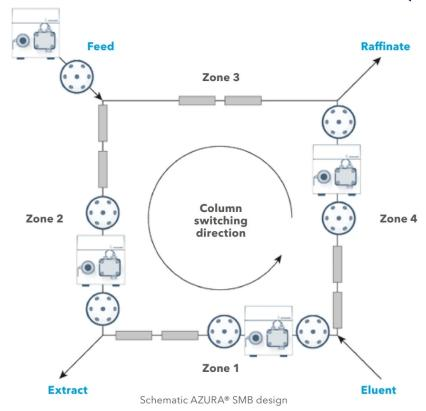
Simulated moving bed chromatography (SMBC) is increasingly applied as a separation technique in the pharmaceutical industry, production of fine chemicals, and in the field of bioengineering.
