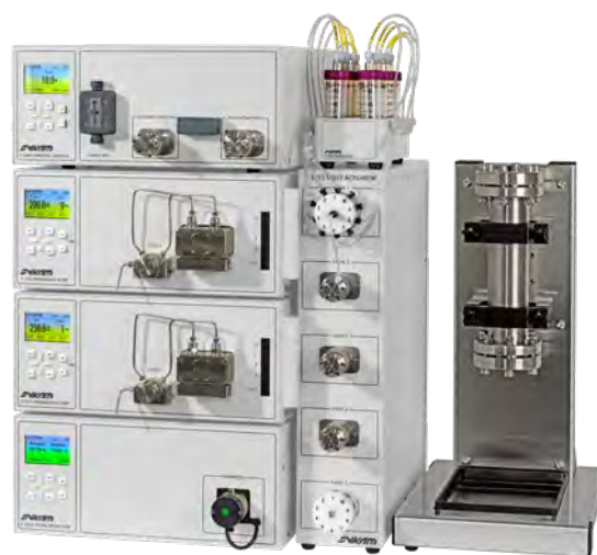
Sykam S 712 binary high pressure gradient HPLC system (stainless steel version)
